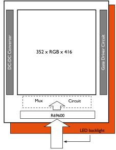
Control Signal, RGB I/F, SPI, VDD, VDDI, backlight
